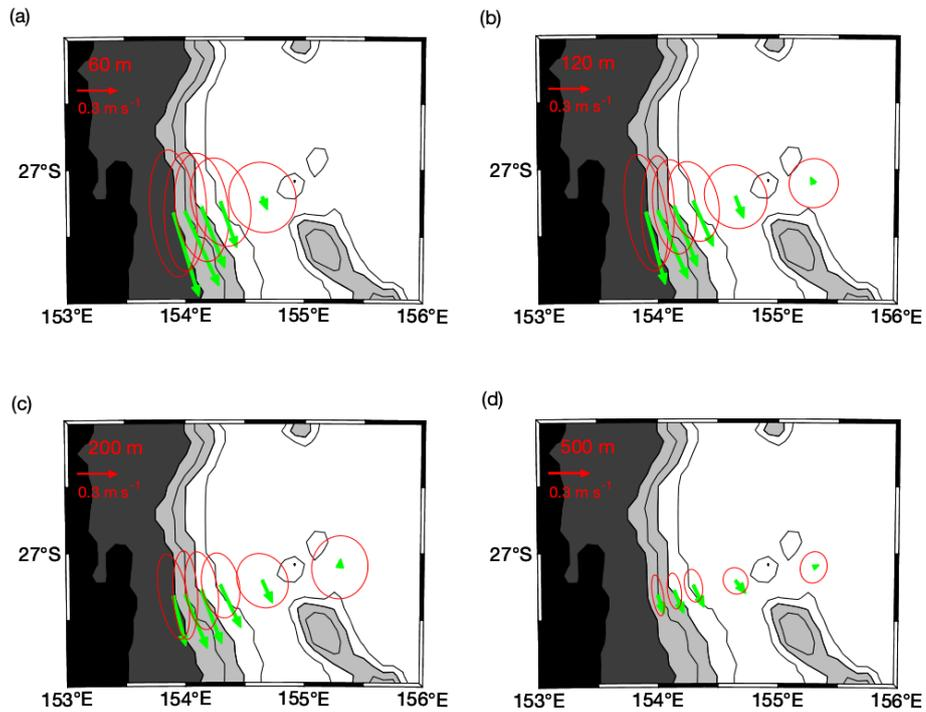
Figure 2. Three-year (May 2015–April 2018) mean along-slope velocity (m/s, green arrow) and velocity variance ellipse (red circle) for (a) 60 m, (b) 120 m, (c) 200 m, and (d) 500 m. The 1000-m, 2000-m, 3000-m, and 4000-m isobaths are contoured and topography shallower than 3000 m is shaded.
