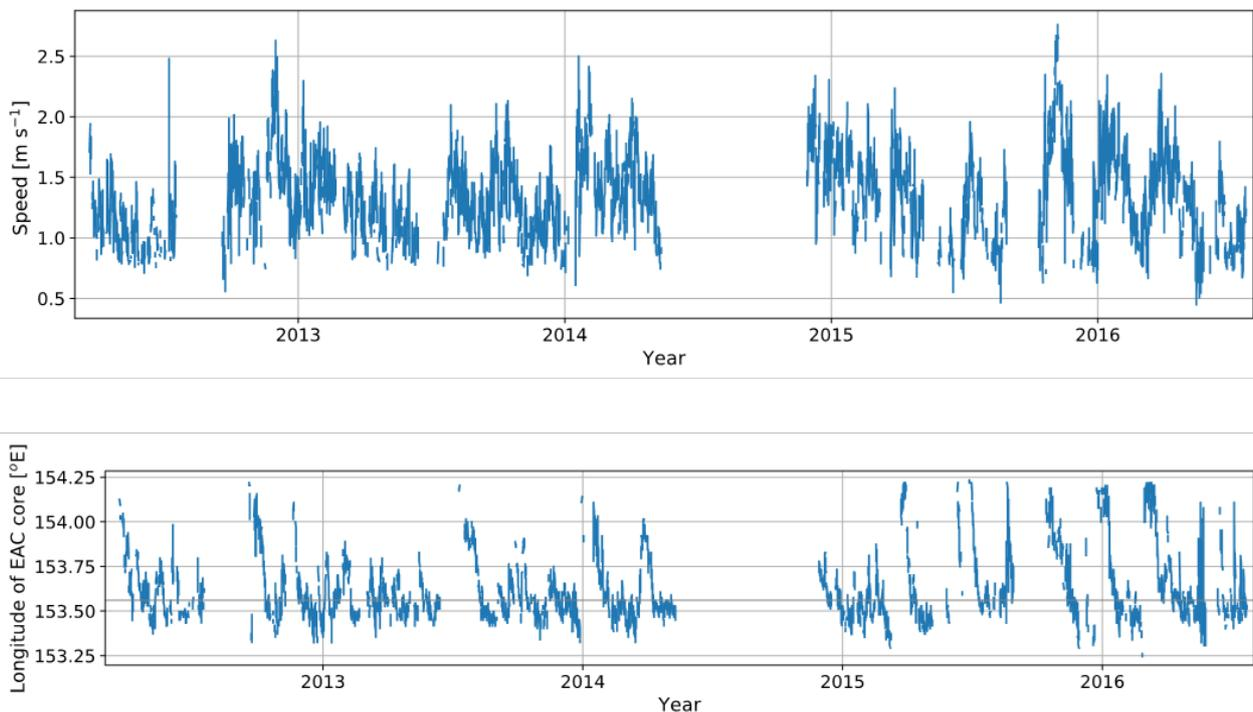
Figure 4. (Top) Speed of the core of the EAC jet calculated from HF radar derived surface velocities centered at 30°S, in a flow following framework (Archer et al. 2017) and (bottom) the position of the core of the EAC jet.
